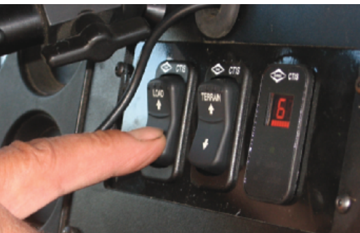
Drivers use two rocker switches to choose Loaded or Empty and On-Road, Off-Road or Emergency. The system then sets pre-programmed tire air pressure, which is shown in a small LED display. Compact control panel is labeled CTI, for Central Tire Inflation, its military name.
