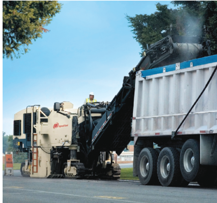
The MT-2000 milling machine features three different drum cutting speeds selectable from the operator’s panel, which Ingersoll Rand says is an “industry-first.”
