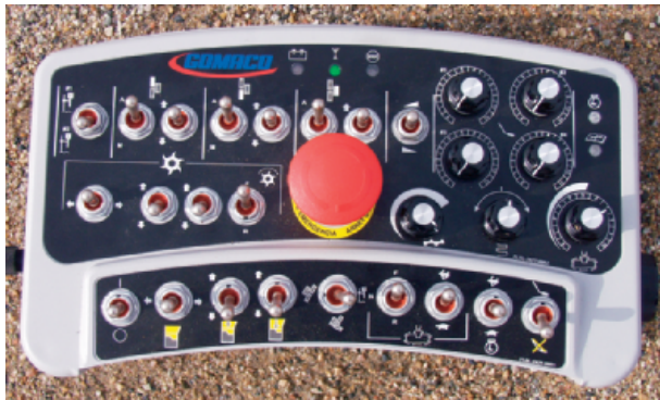
The 11-inch-wide control handset offers the operator full paving control, with 21 toggle switches, three control dials, five indicator lamps, and four variable controls for vibrator circuits.
